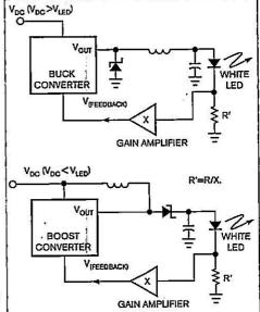
Figure 2 In these circuits, an amplifier gain reduces the power dissipated in the series resistor by a factor equal to the gain.
