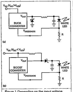
Figure 1 Depending on the input voltage, buck (a) or boost (b) regulators drive high-intensity white LEDs.
